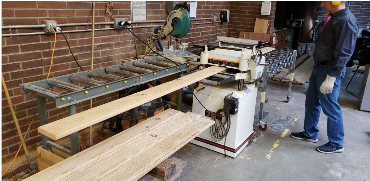
Figure 1: planing of lamellas
