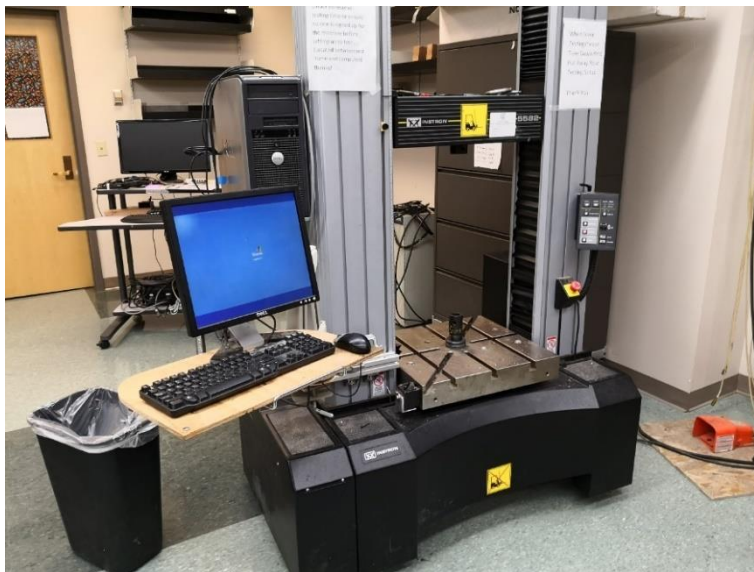
Figure 8: Universal Testing System – Instron 5582 Source: (separate figure, 2020)
