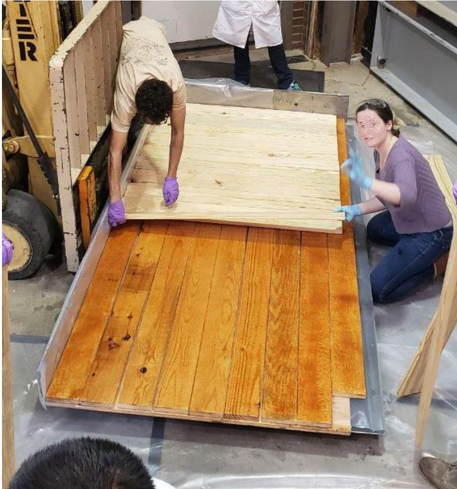
Figure 4: board layup Source: (SOP for CLT fabrication, 2018)
