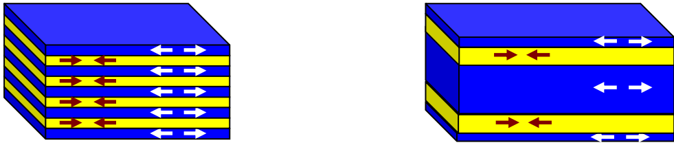
a) b) Figure 6: Schematic of a) Periodic design (9 layers), b) non-periodic design (5 layers)
