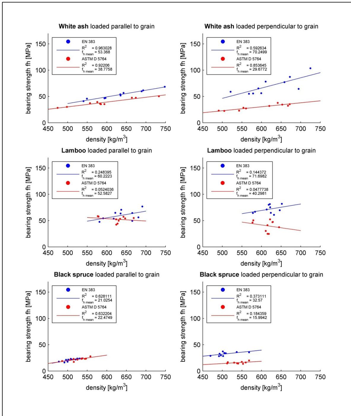
Figure 4-6: Comparison EN 383 and ASTM D 5764 – bearing strength over density
