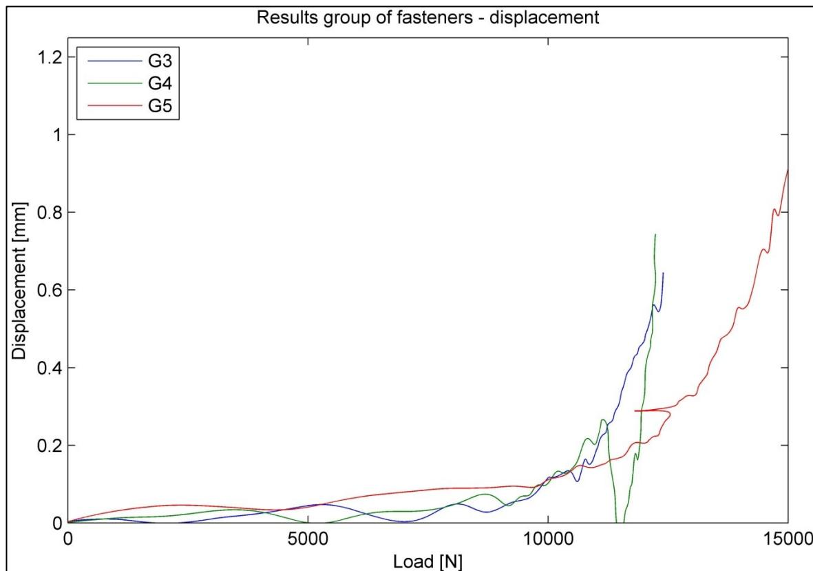
*Figure 5-6: Results group of fasteners – displacement*
