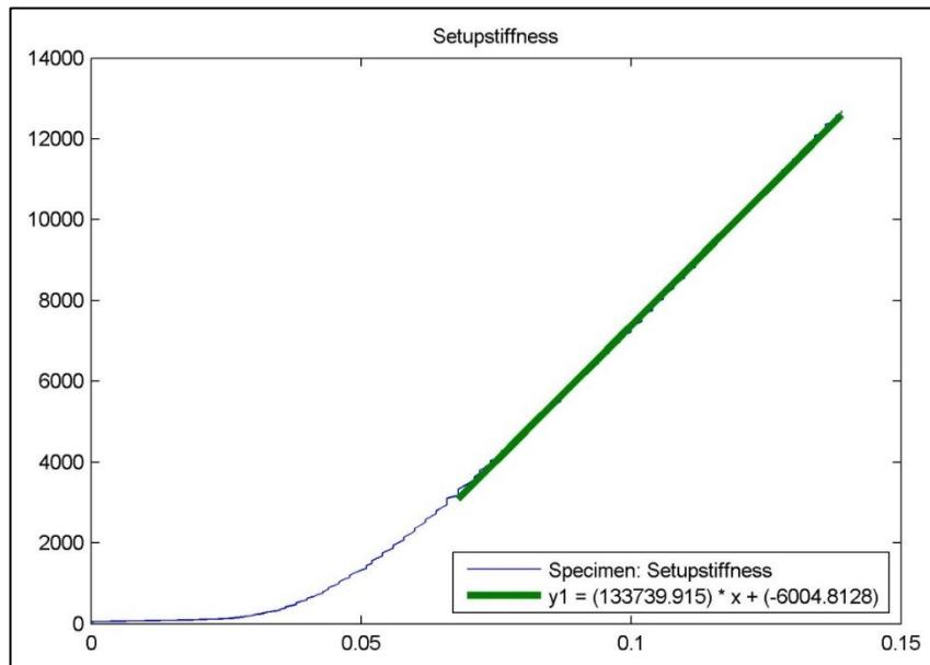
Figure 4-4: Setup stiffness
