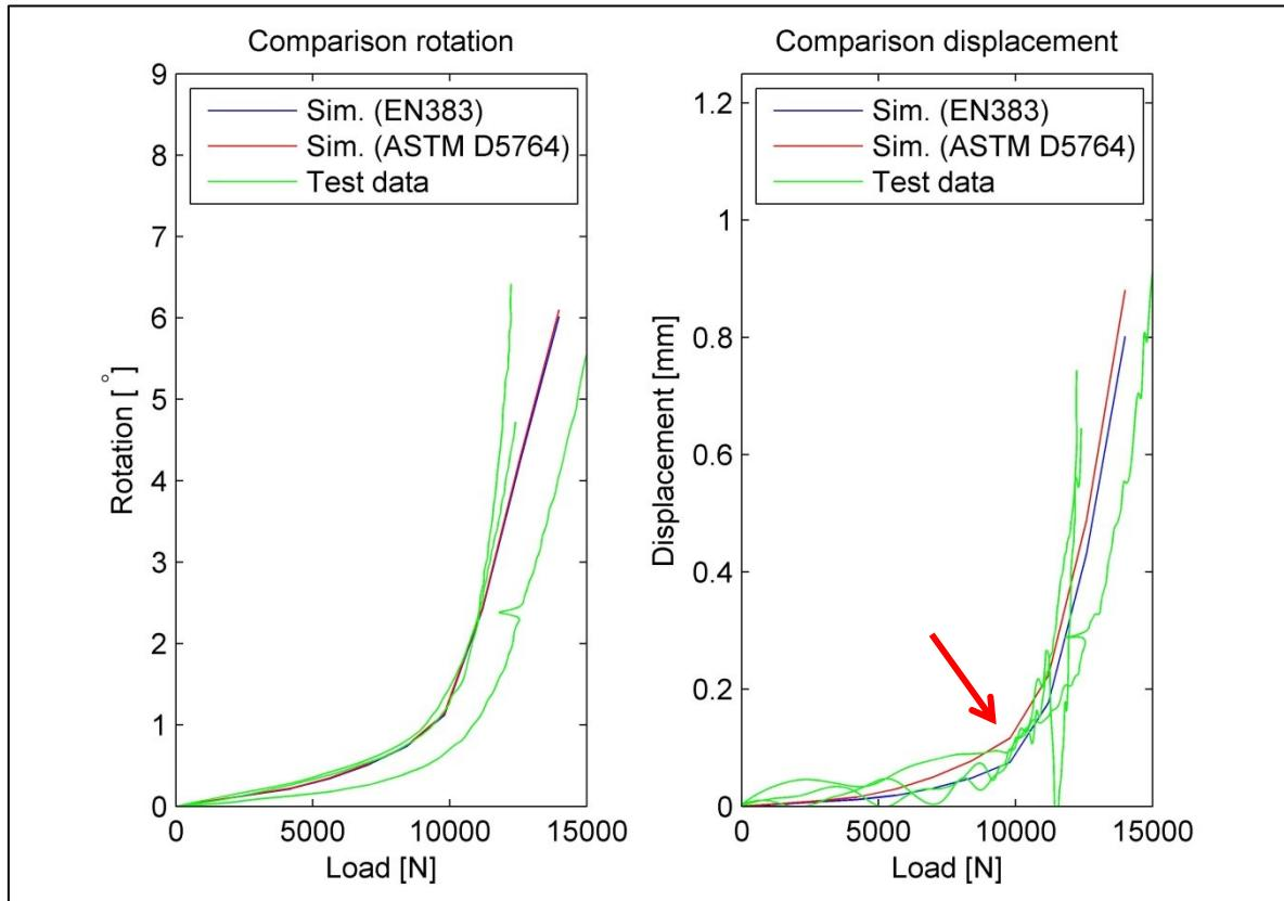
*Figure 5-16: Comparison Simulation data and Test results for mean density – calibrated*
