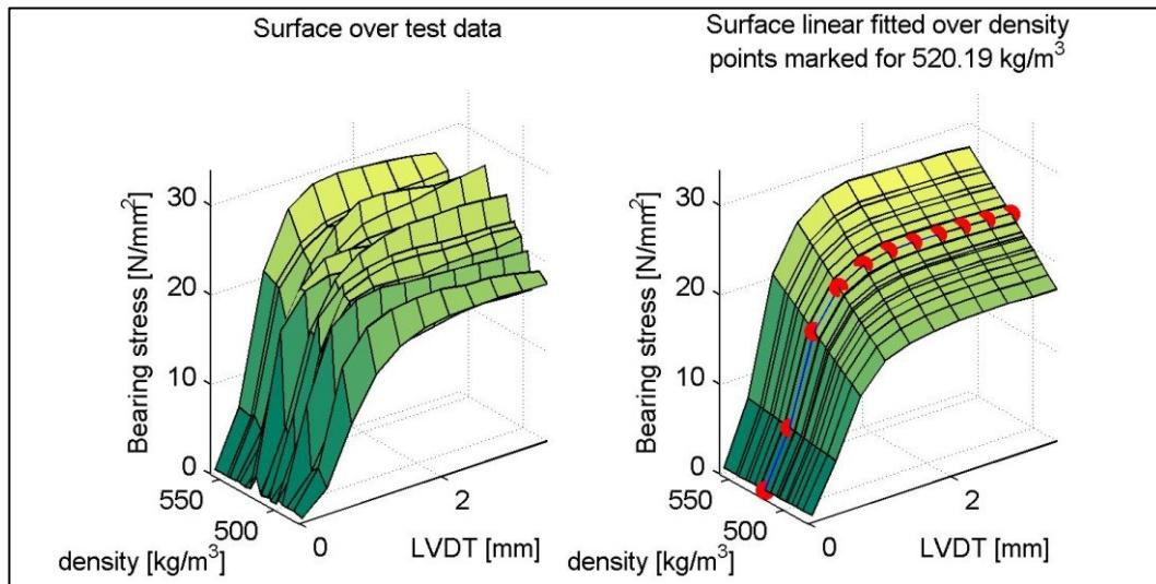
Figure 4-7: LDD surface parallel to grain - EN 383
