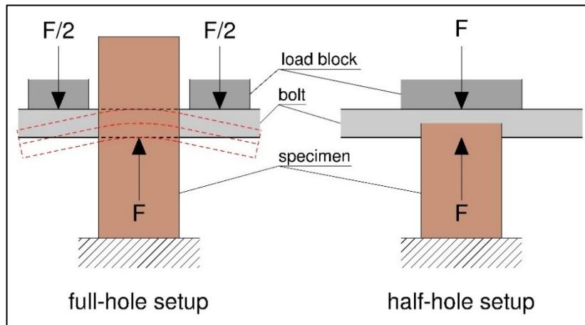
Figure 2-5: Deformation of loaded bolt
