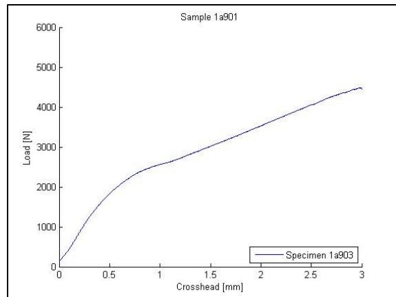
Figure 1-3: Typical load-displacement curve - loaded perpendicular to grain
