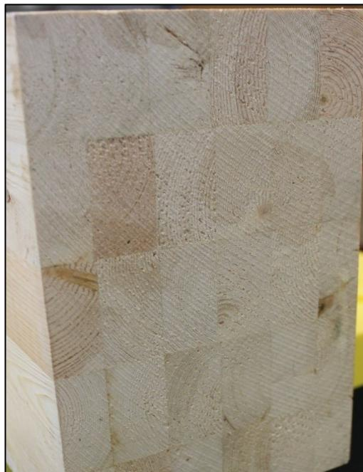
*Figure 3-4: Structure of glulam beam*
