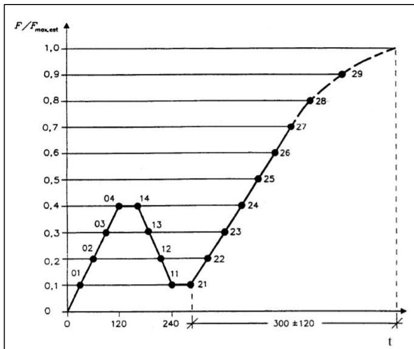
Figure 2-8: EN 383 loading cycle [5]
