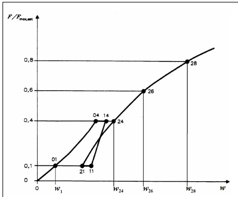
Figure 2-10: Idealized load-displacement curve according to EN383
