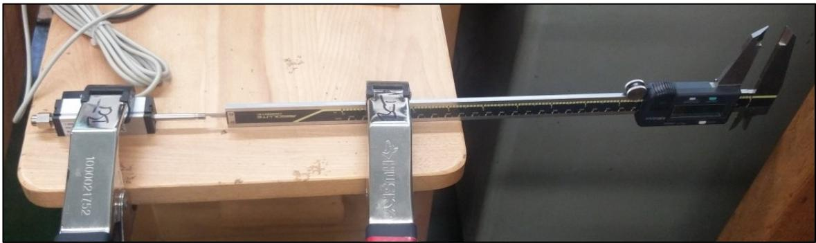
Figure 3-5: LVDT calibration setup
