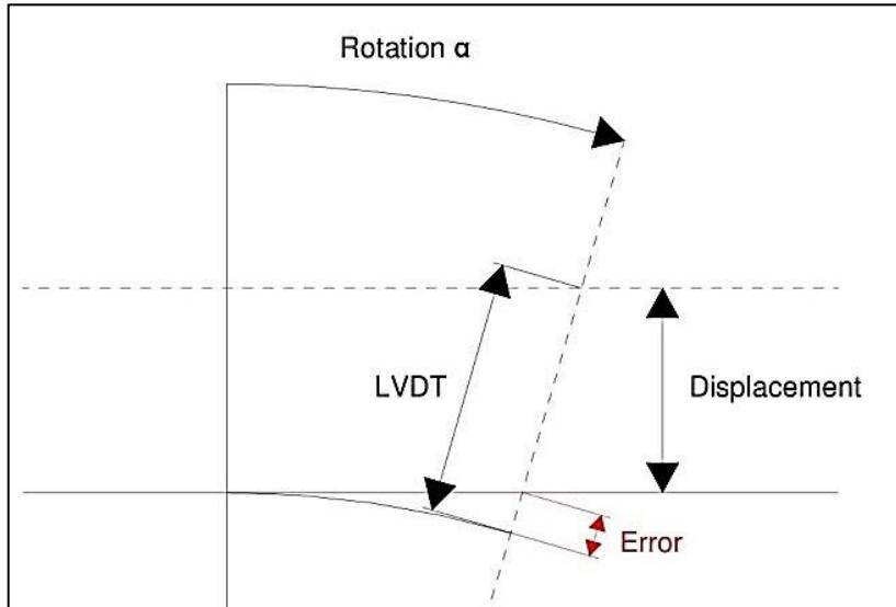
Figure 5-5: LVDT Error due to rotation; upper LVDT
