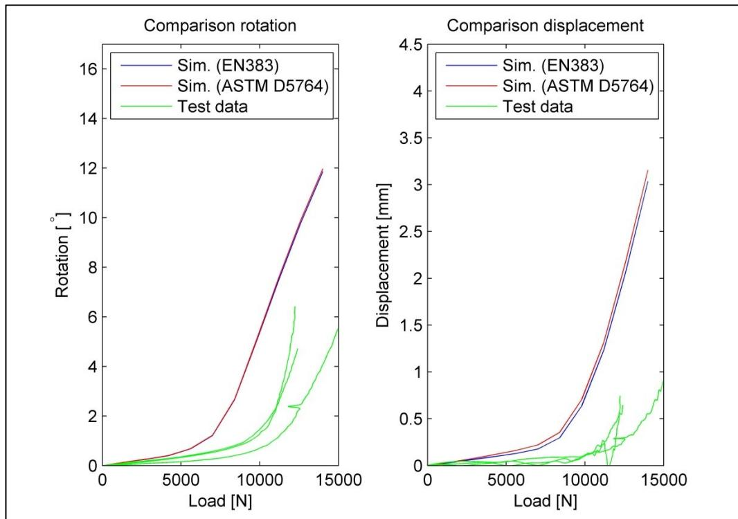
*Figure 5-13: Comparison Simulation data and Test results for mean density – uncalibrated*
