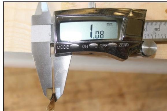
*Figure 5-15: Measurement of the matrix-thickness*
