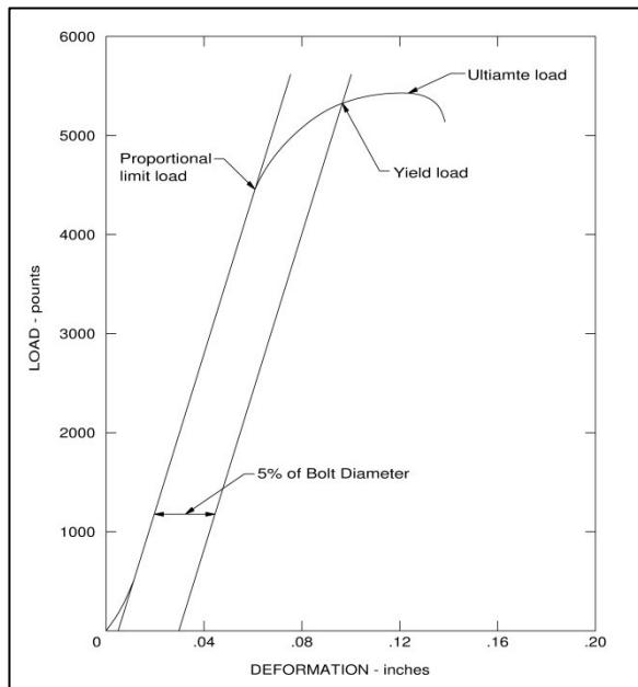
Figure 2-9: ASTM D 5764 yield load [6]
