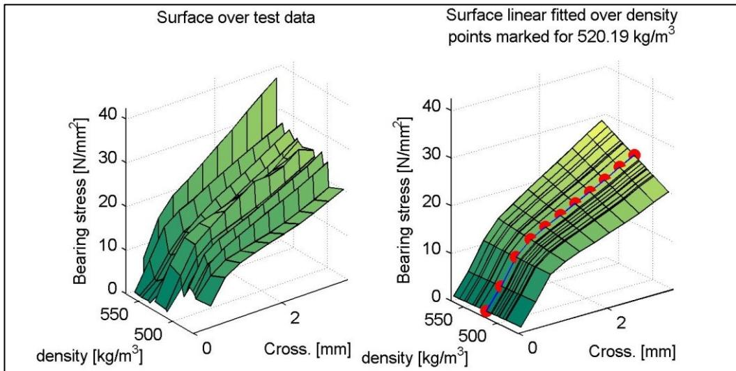
Figure 4-10: LDD surface perpendicular to grain - ASTM D 5764
