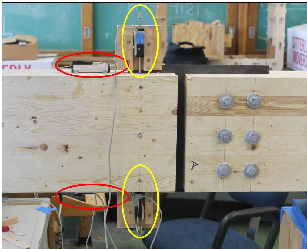
Figure 5-2: Connection with added LVDTs
