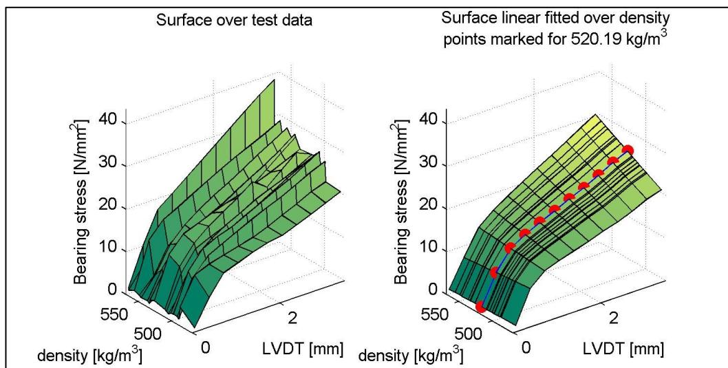
Figure 4-8: LDD surface perpendicular to grain - EN 383
