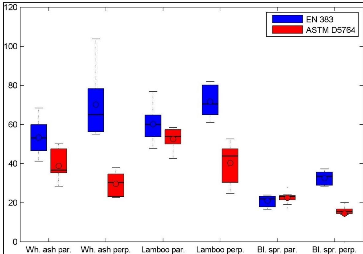
*Figure 4-5: Results - comparison statistics of bearing strength [N/mm<sup>2</sup>]*
