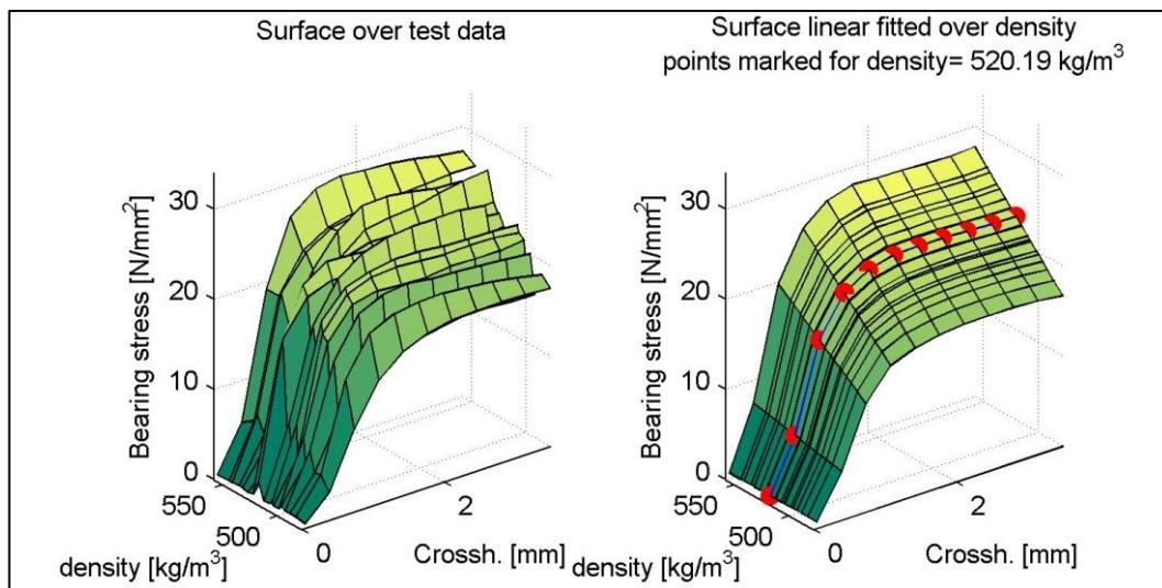
Figure 4-9: LDD surface parallel to grain - ASTM D 5764
