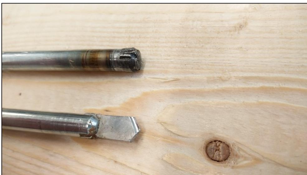
Figure 5-1: Broken drill-tip
