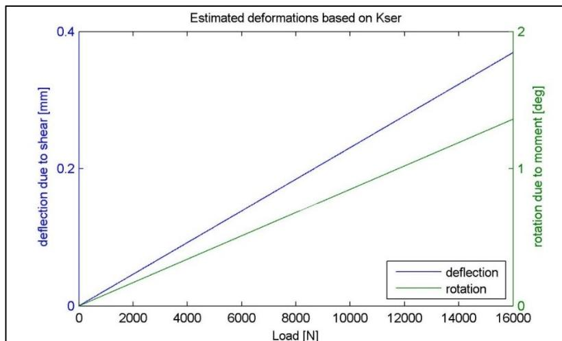
Figure 3-11: Deflection and rotation estimated according European code
