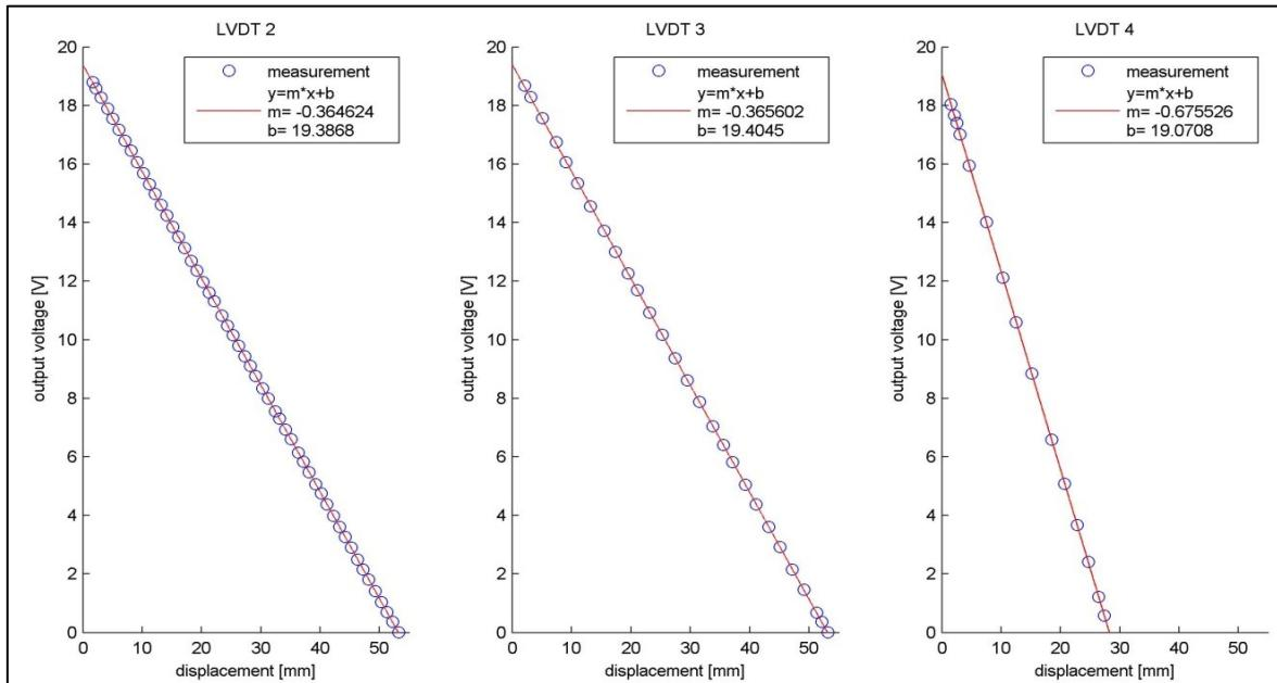
Figure 3-6: LVDT calibration results
