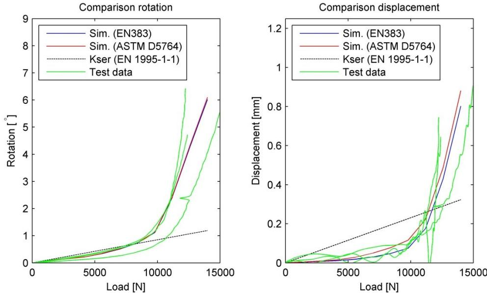
Figure 5-17: Comparison of test data, simulation and approach with  $K_{ser}$
