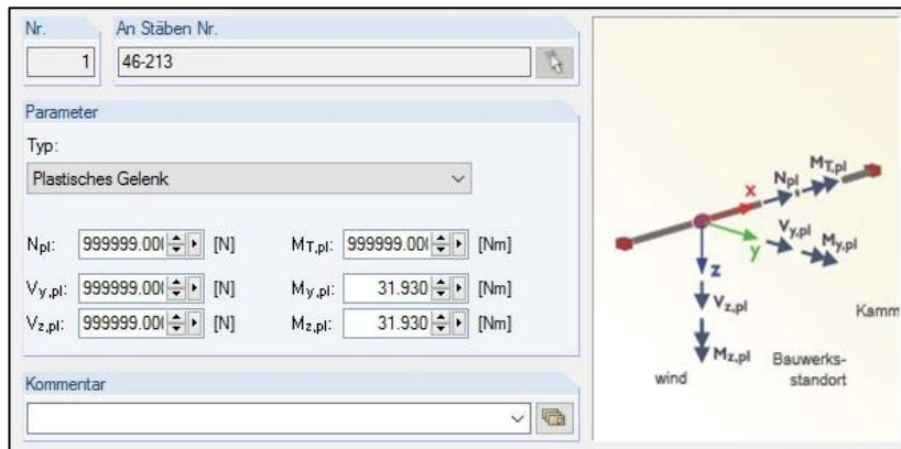
Figure 5-9: RSTAB - Settings for plastic hinges<sup>9</sup>
