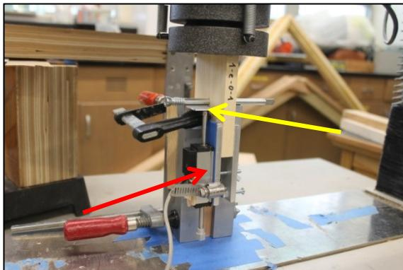
*Figure 4-2: LVDT assembly (a)*
