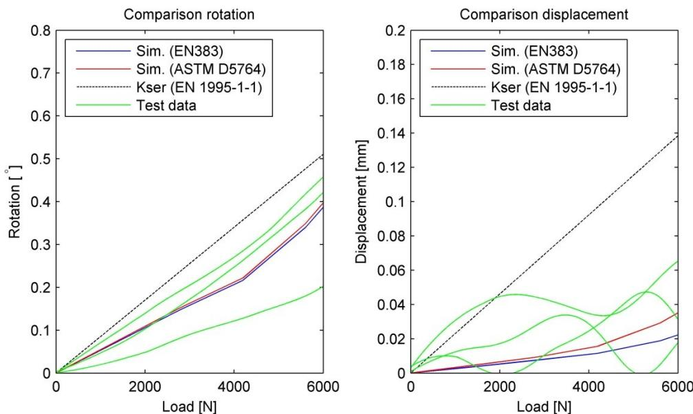
Figure 5-18: Comparison of test data, simulation and approach with  $K_{ser}$
