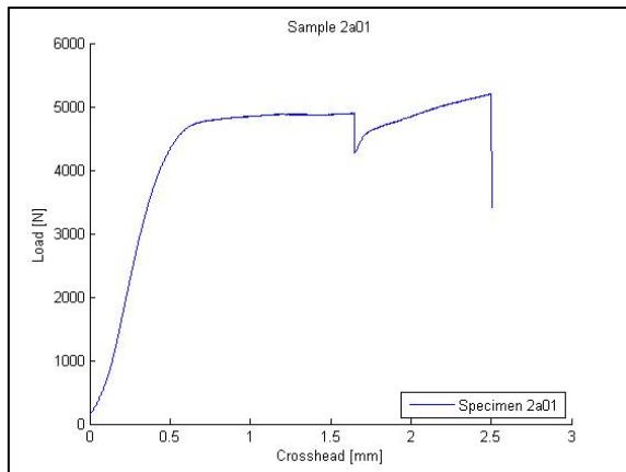
Figure 1-2: Typical load-displacement curve - load parallel to grain
