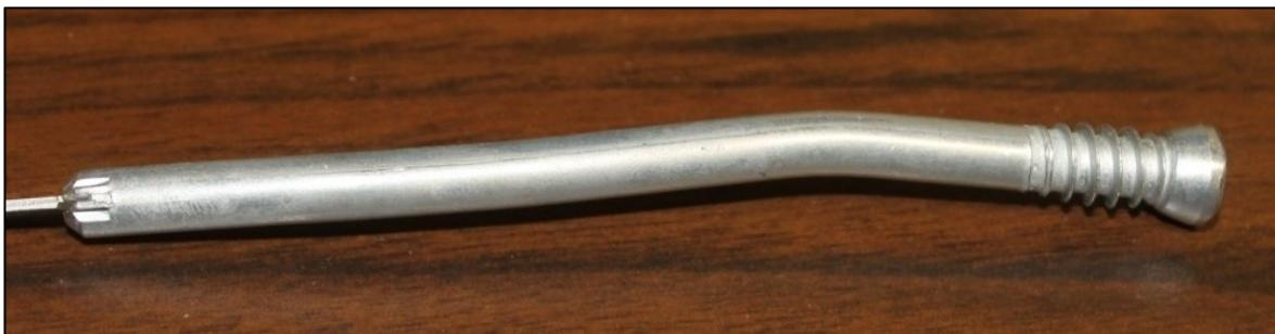
Figure 4-1: Destroyed bolt after pretests
