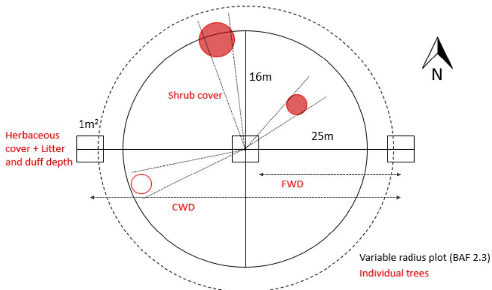
Figure 4. Plot design. Individual trees are represented as red circles: filled ones would be tallied, empty one would be out. FWD was measured on a 12.5m transect, CWD on a 25m transect. Shrub cover was estimated within a fix area plot of 8m radius (200m<sup>2</sup>). Herbaceous cover and litter and duff depth were estimated three times along a 25m transect, in a 1m<sup>2</sup> subplot.
