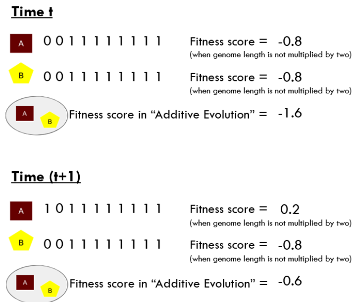
Figure 4.4: Unwanted evaluation of the genomes. A tail-end one leads to a fitness decrease of \frac{1}{10} = 0.1 .
