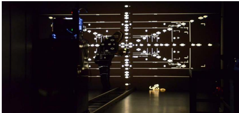
Figure 11. Lenses being checked on a Gecko-Cam Lens Projector in a large projection room. The prototypes looked contrasty, very sharp (high resolution), with very straight geometry. Same lens charts are being used by VFX teams (Fauer, 2015).
