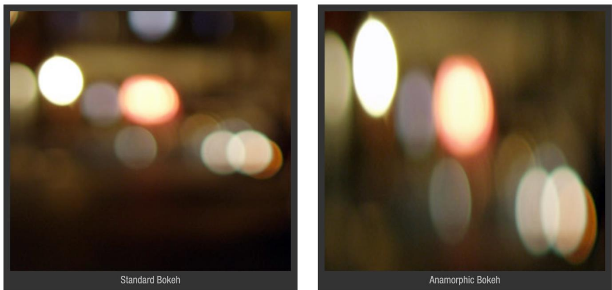
Figure 6. Comparison between bokeh from a spherical lens(left) and an anamorphic lens(right). Pictures taken on a RED digital camera (RED, n.d.).
