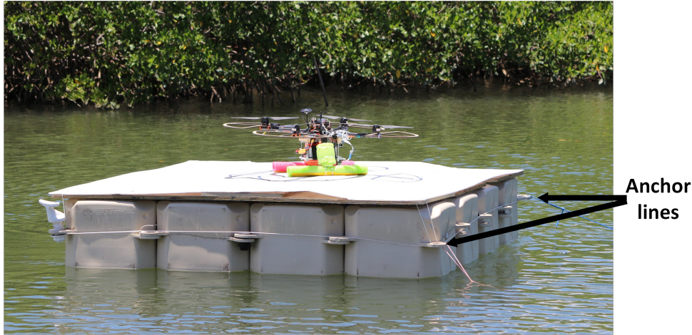
Figure 3.12: Test setup on water. The landing target is mounted to floating dock units and held in place by two anchors. The anchors are attached to the blue and pink ropes attached to the corners of the floating dock.
