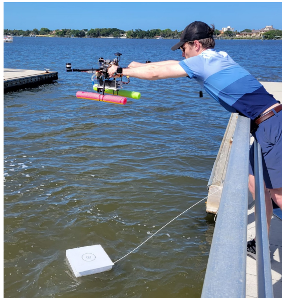
Figure 3.1: Collecting sample data on a scaled-down platform to validate the image recognition algorithm.
