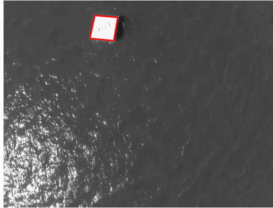
Figure 2.14: Fitted contours using thresholded image and checking if the contours have the right parameters. For easier viewing the contour is superimposed on the grayscale image.
