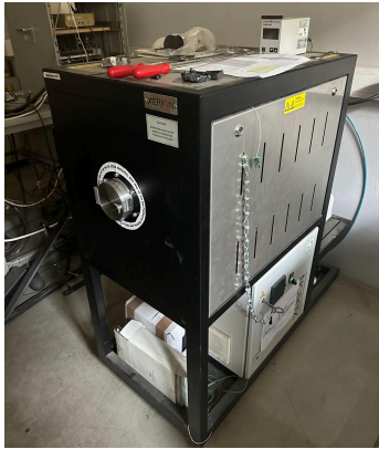
Figure 23. Furnace setup for heat treating the F82H cantilevers.
