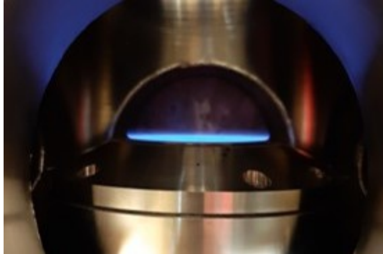
Figure 1.1: Laminar and premixed flat flame ( CH_4 with 21 vol.% O_2 ) above the surface of the FFB.
